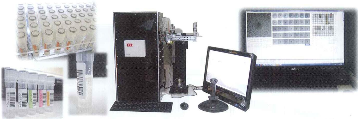
**AutoMODS** is a system of TB culture testing with liquid media allowing simultaneously identification of TB strains and drug susceptibility/resistance with a comparable quality to reference system. AutoMODS system is composed of a digital microscope, a 3 axis moving table, an incubator, a computer and software, and liquid media in tubes.
